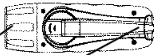
Fold-out Handle drives internal generator which charges the internal NiMh storage cells
